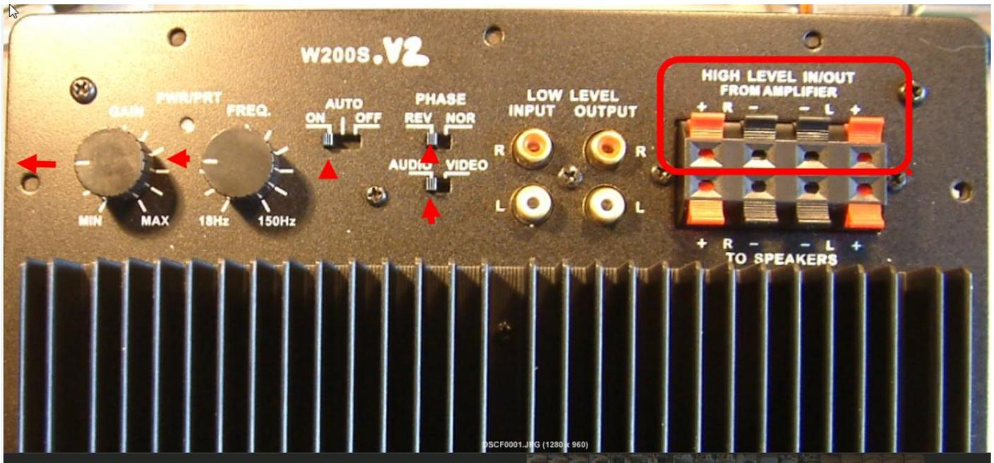
**HIGH LEVEL IN:** HOME THEATRE and STEREO AUDIO SETTINGS FOR BEST SOUND --- Using speaker cable high level input to subwoofer amplifier.
