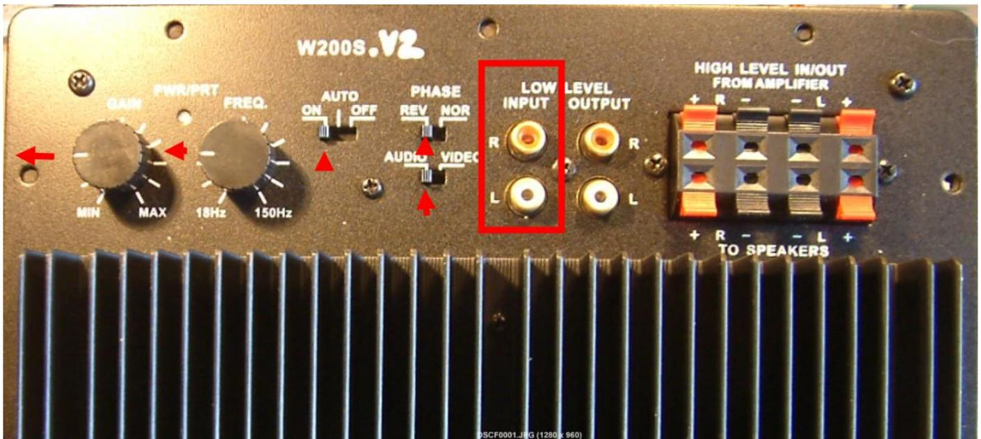
RECOMMENDED SETTINGS FOR BEST SOUND using an RCA cable from the Sub Out on Home Theatre receiver connected to the LOW LEVEL inputs of the S200W-V2 Subwoofer amp
